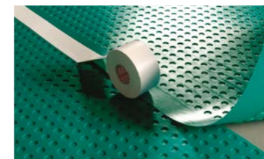
Moisturbloc Extreme™ PGUDLMOI15, 1.05 x 15 m = 15 m² (5 cm overlap) Three times the moisture resistance of traditional PE film. Can be installed on concrete floors with up to 95% relative humidity. Ideal in basements and on concrete floors with high humidity. Makes it possible to install floors earlier during the construction of new-builds. Thickness: 2.5 mm. Material: Polypropylene. Tape included.
